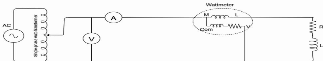
Fig. No. 10.1 : Circuit diagram for measurement of power and power factor with R-L Load.
