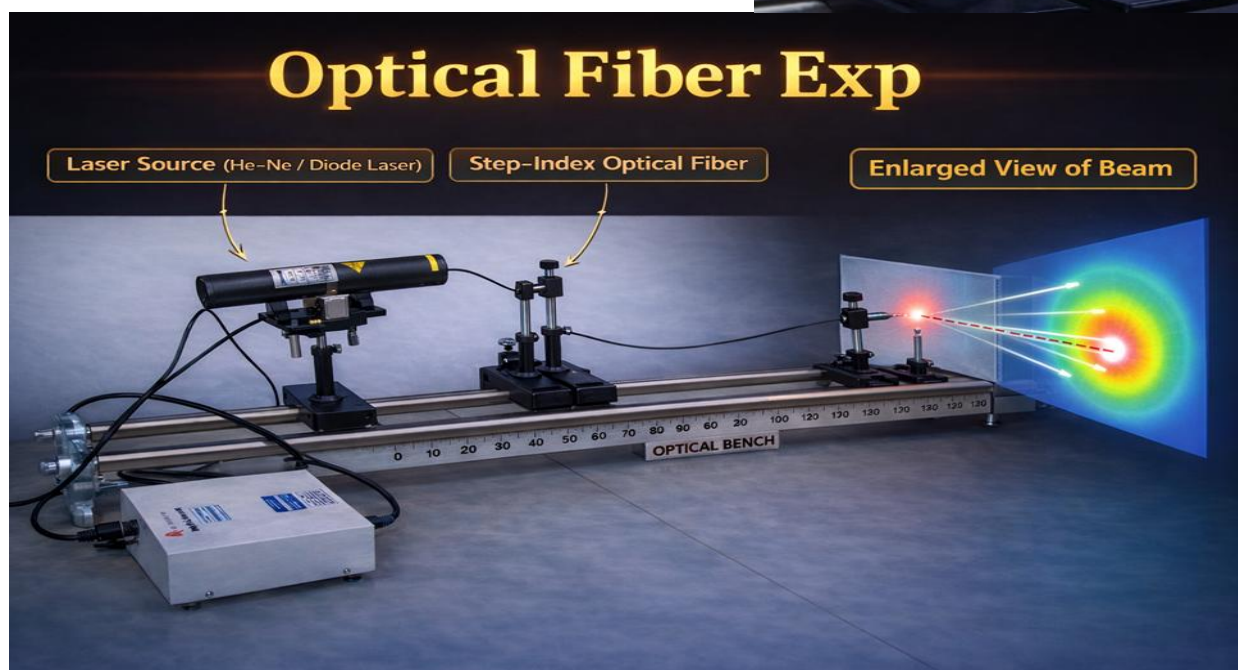
Fig. 11.01: Experimental Setup for Numerical Aperture Measurement
