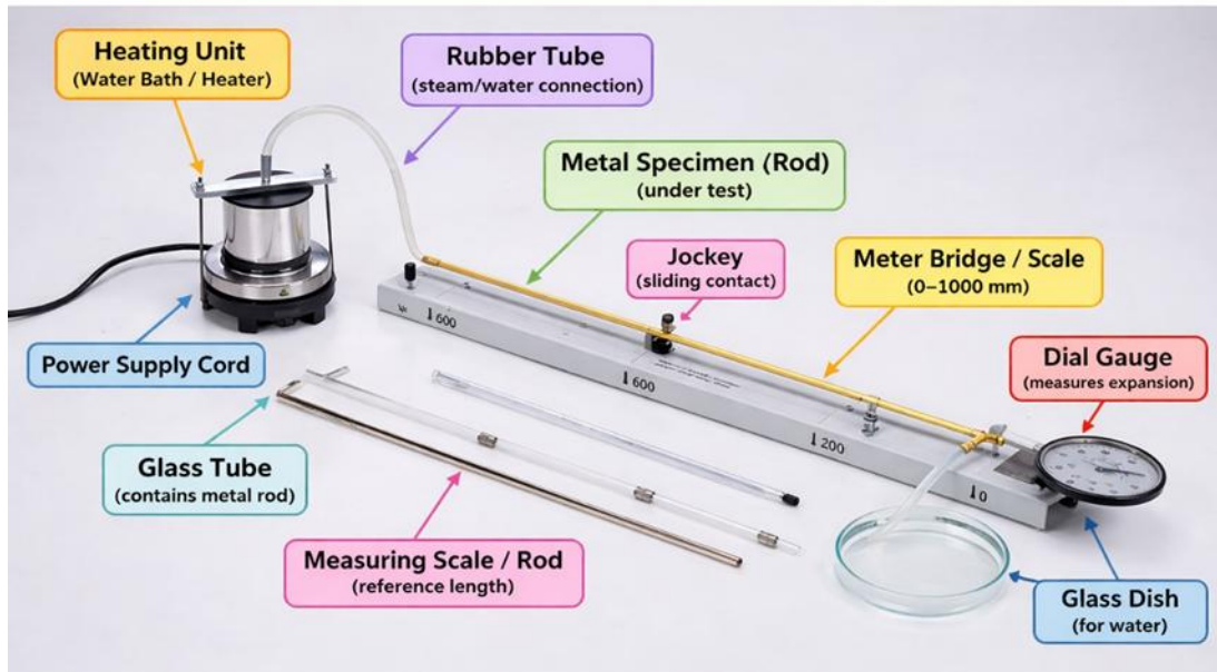
Fig:07.01 Pullinger's apparatus for measurement of Coefficient of Linear Expansion
